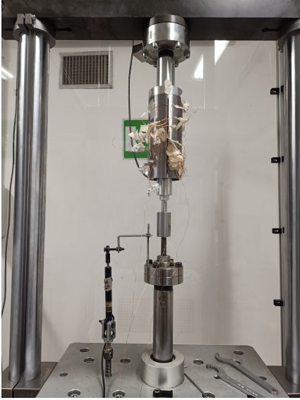
(a) Regenerator prototype and displacement sensor mounted on the test-rig.
