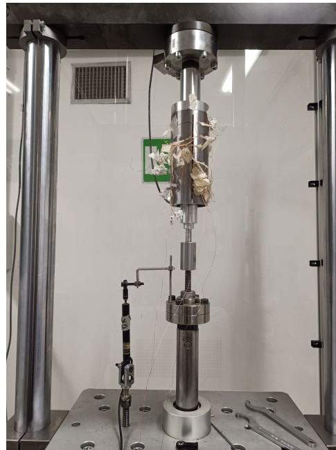
(b) Regenerator prototype and displacement sensor mounted on the test-rig.
